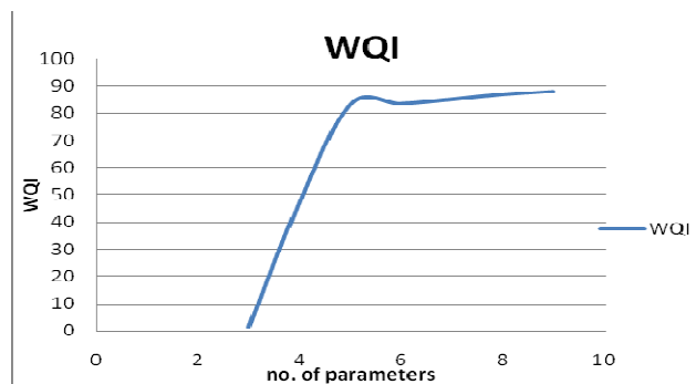
Figure 3.6: Impact on WQI on Removing Pollutant with Low Quality Factors (Eq. 4)
