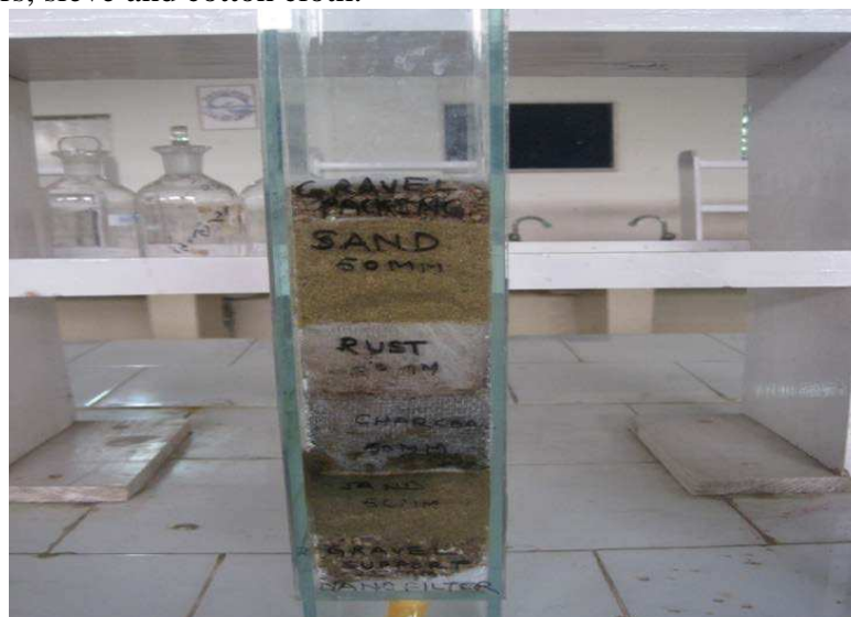
Fig2. Showing a Full Setup of Rust Column (Source: Picture taken from camera: Self)
